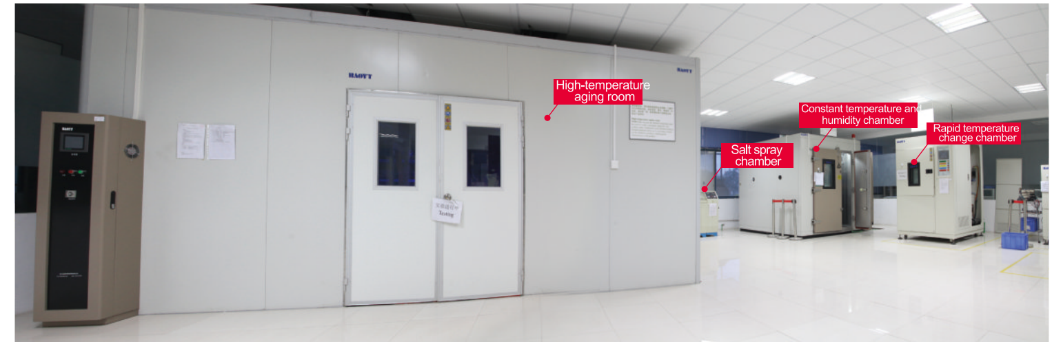
Climate Environmental Laboratory Simulate various extreme climate environments to ensure the quality of products.
